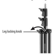
2 Pull outward on the legs. Set upright, then push down on the legs and tighten the leg locking knob.
